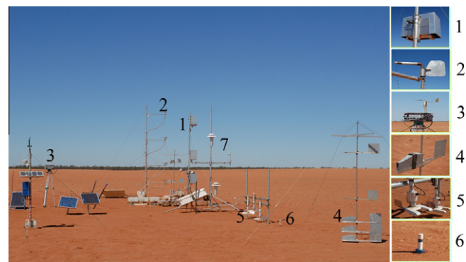
Fig. 19. An example for the set up of a wind-erosion monitoring system in field. Dust concentrations and sizedistributions are measured using Optical Particle Counters (1, OPC at 1, 2 and 3.5 m); TSP concentrations are measured using high-volume air samplers (2, TSP at 1, 2, 3.5 and 5 m) and PM10 concentrations are measured using a Dust Track (3, at 2m); Saltation flux is measured using an array of Fryrear sand traps (4, at 0.1, 0.2, 0.5, 1 and 2 m), Sand Particle Counters (5, SPC at 0.05, 0.1 and 0.3m) and a Sensit (6, at 0.1 m). It also consists of a micro-meteorological station for recording wind profiles and other meteorological data (7, AWS). (Experiment set up by M Mikami, J F Leys and M Ishizuka).
