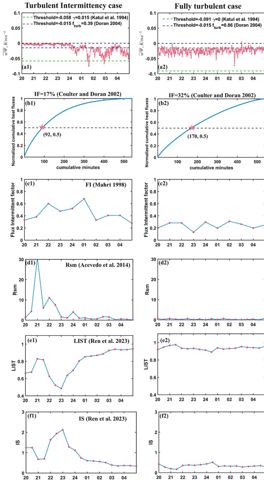
Fig. 6. Different indexes characterizing turbulence intermittency in turbulent intermittency case and fully turbulent case. (Reproduced from Ren et al., 2023b).
