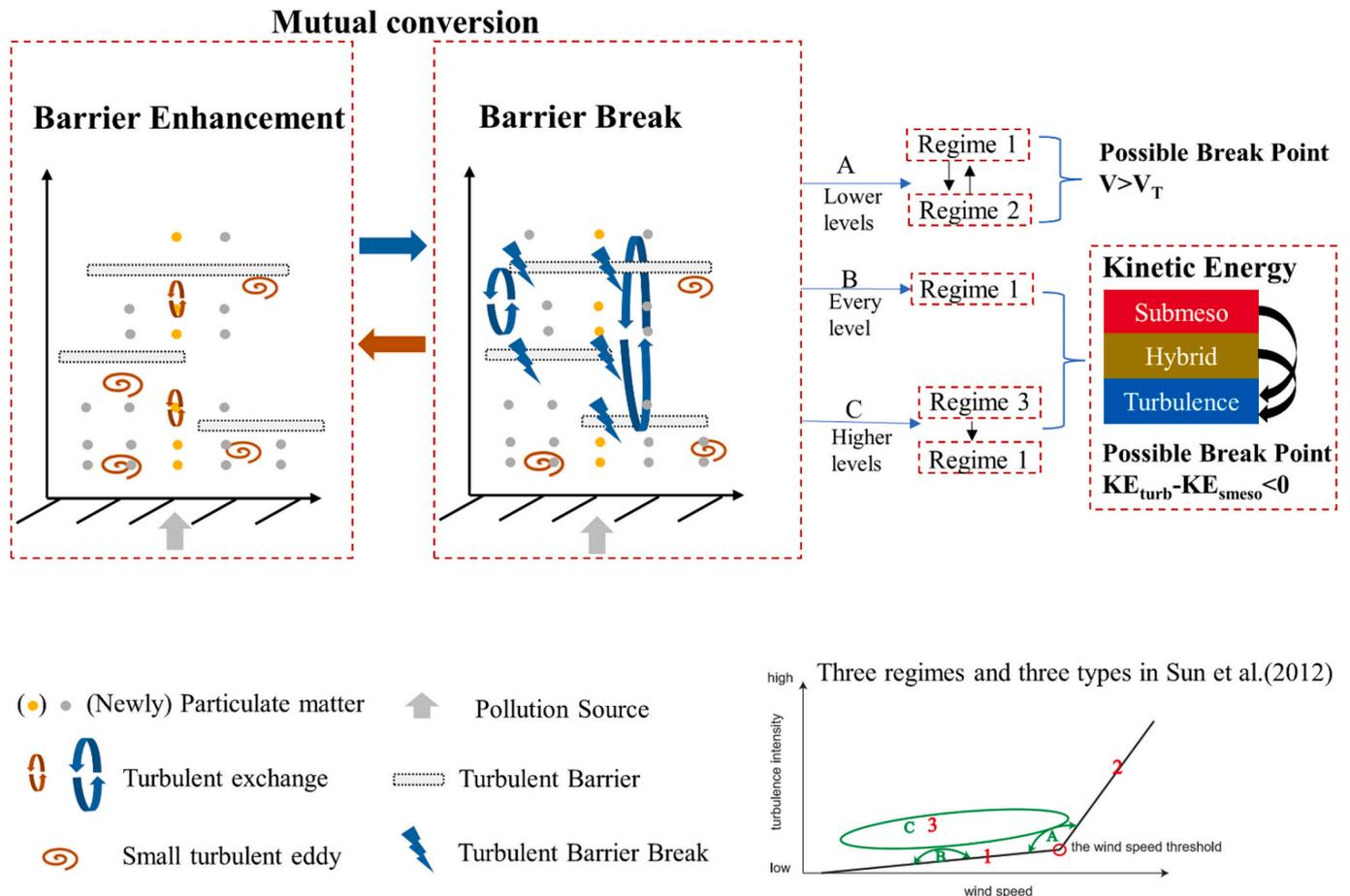
Fig. 10. Schematic of the characteristics of turbulence barrier enhancement and break, the energy transition and possible breakpoint for different turbulence intermittency types. (Cited from Ren et al., 2023c).
