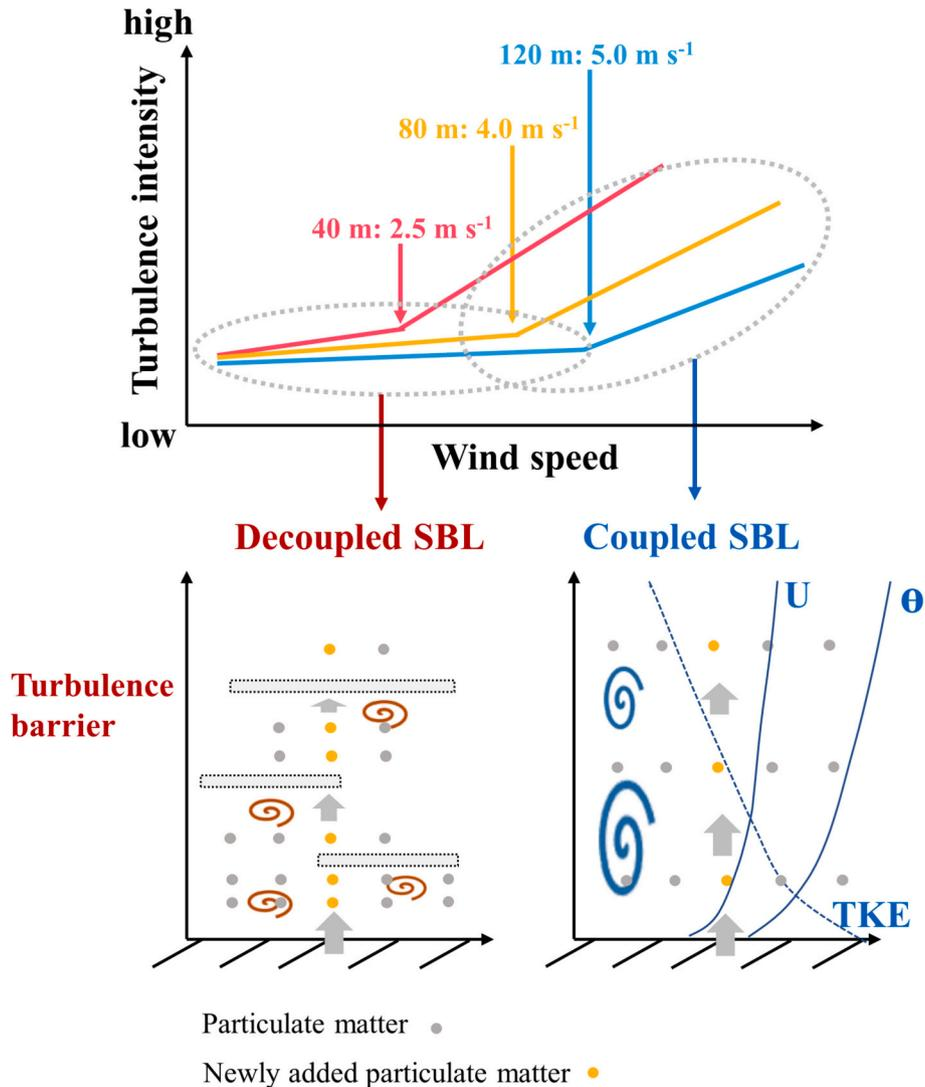
Fig. 1. Schematic of the distinctly different turbulence structures, pollutant transportation rate, and distributions of coupled and decoupled SBLs. (From Ren et al., 2023a).
