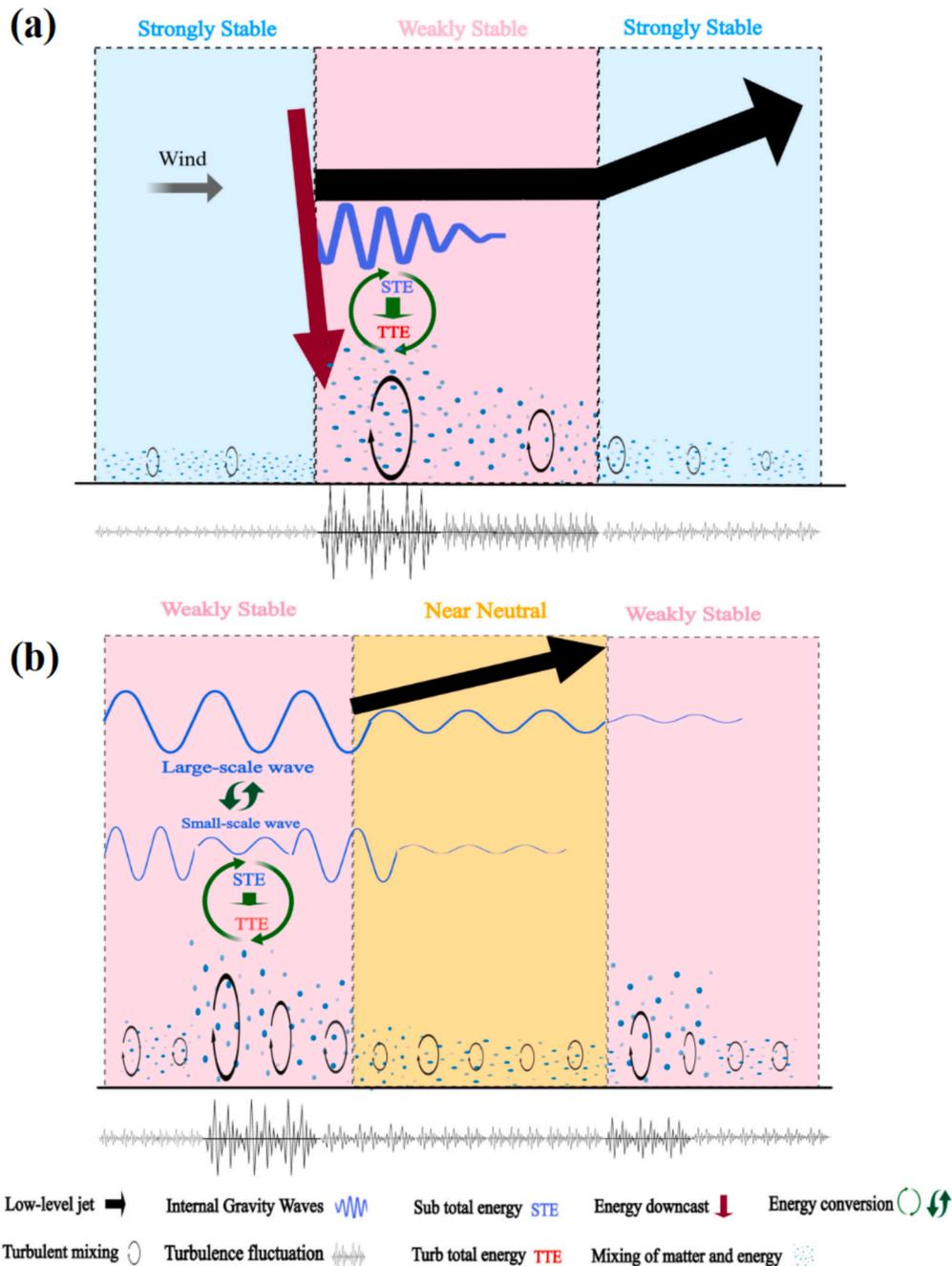
Fig. 4. Schematic representation of the mechanism of the effect of the interactions between low-level jets (LLJ) and internal gravity waves (IGWs) on the boundary layer turbulent structure: (a) case with a lower-positioned, long-duration, stronger LLJ interacting with short-duration, stronger IGWs; (b) case with a higher-positioned, short-duration, weaker LLJ interacting with longer-duration, weaker IGWs. (Cited from Ding et al., 2024).
