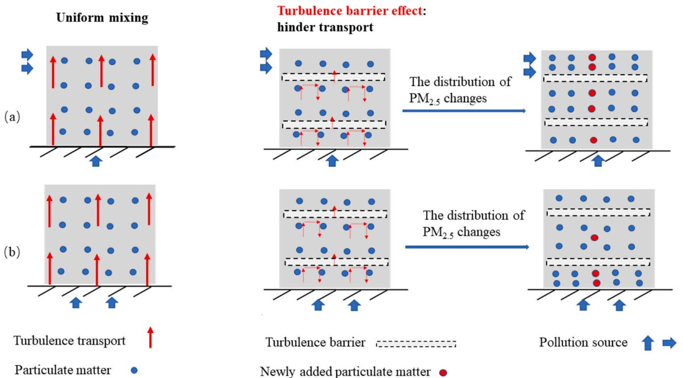
**Fig. 9.** Schematic of how the turbulence barrier effect hinders transport and is helpful for the accumulation of  $PM_{2.5}$  in the surface layer. The first row shows the situation of relatively low emissions from ground sources and relatively high pollution at high altitudes from regional transport. The second row shows a simpler and more universal situation where only ground sources exist. (Cited from [Ren et al., 2021a](#)).
