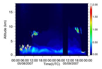
**Figure 4.** MPL normalized relative backscatter at SACOL for 8 and 9 May 2007.
