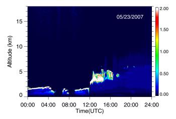
**Figure 9.** MPL normalized relative backscatter intensity at SACOL for 23 May 2007.
